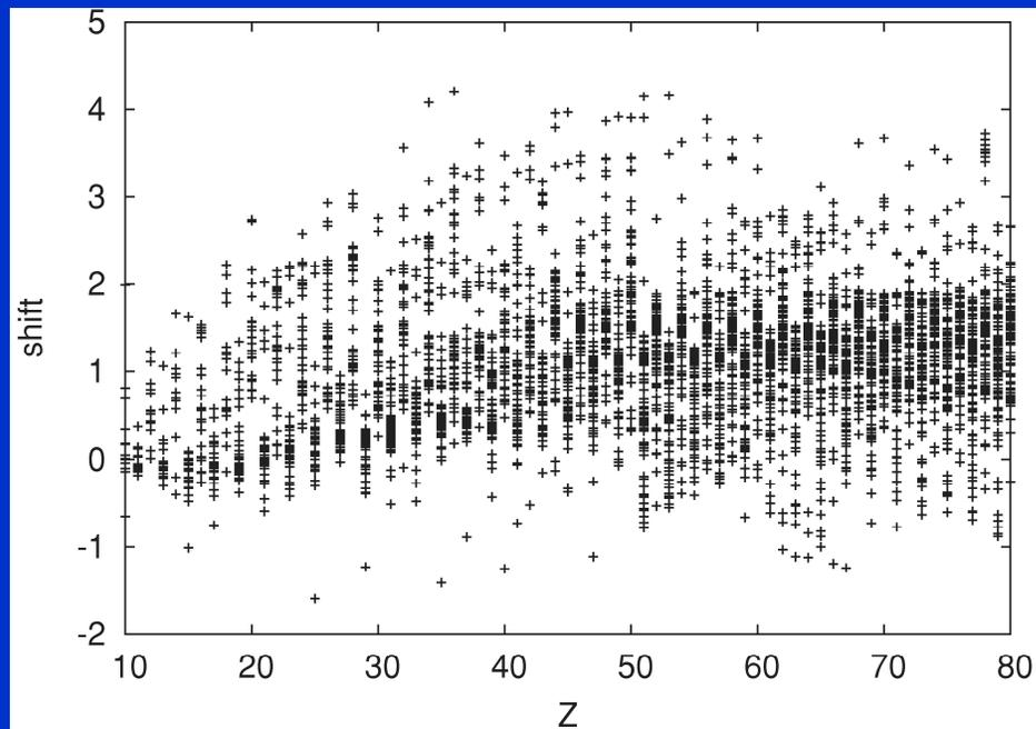
FIG. 8. Shifts  $\delta$  (MeV) of the maximum of the integrand relative to  $E_0$  of the Gaussian approximation as a function of the target charge  $Z$  for  $(p, \alpha)$  reactions at  $T = 5$  GK. The shifts are larger as for  $(\alpha, p)$  reactions and they are positive.
