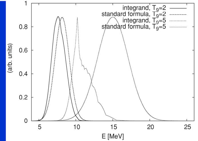
FIG. 6. Comparison of actual reaction rate integrands  $\mathcal{F}$  and Gaussian approximations of the Gamow window for the reaction  $^{169}\text{Tm}(\alpha,\gamma)^{173}\text{Lu}$  at  $T = 2$  and  $5$  GK. The integrands and Gaussians have been arbitrarily scaled to yield similar maximal values. While the integrand is still for  $T_9 = 2$ , it is about  $5$  MeV at  $T_9 = 5$ . Also, the integrand can be clearly seen at  $T_9 = 5$ .
