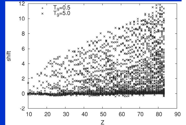
FIG. 11. Shifts  $\delta$  (MeV) of the maximum of the integrand relative to  $E_{MB}$  as a function of the target charge  $Z$  for  $(n,p)$  reactions at two temperatures. Almost no shift is observed at  $T_9 = 0.5$  but shifts become large at  $T_9 = 5.0$ .
