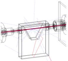
The **transmission** of the recoils and the **efficiency** of the BGO array of DRAGON were studied with the GEANT3 toolkit.
