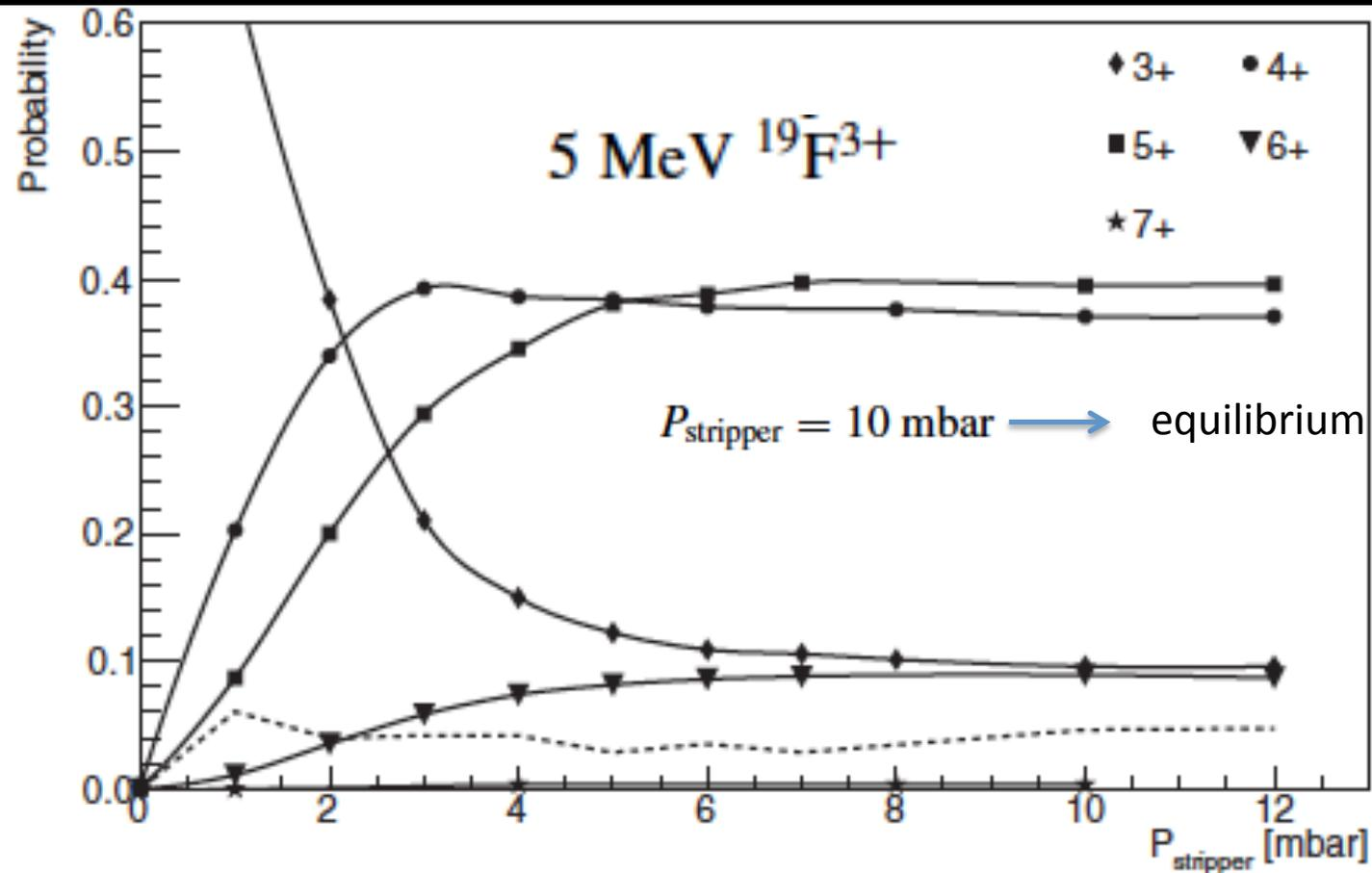
FIG. 4. Charge state probability of  $^{19}\text{F}$  ions as a function of the Ar post-stripper inlet pressure  $P_{\text{stripper}}$  at 5.0 MeV beam energy. Lines connecting the points are to guide the eye only. The dotted line represents the unmeasured current at this energy, due to nonaccessible 1+, 2+ charge states and further charge exchanging in the CSSM chamber; see text for details.
