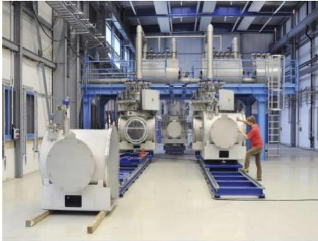
GSI: Series test facility for the SIS100 s.c. dipole magnets, string test, current leads and local cryogenics components.
