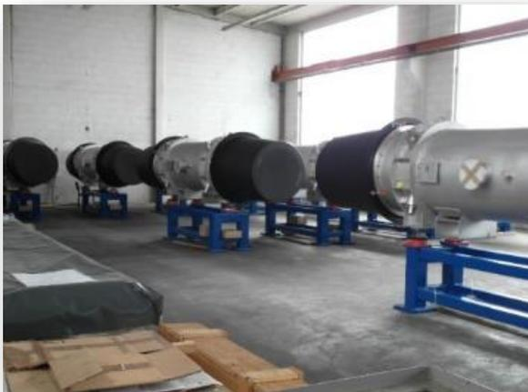
SIS100 quadrupole units shipped from JINR to BNG for integration into FOS module
