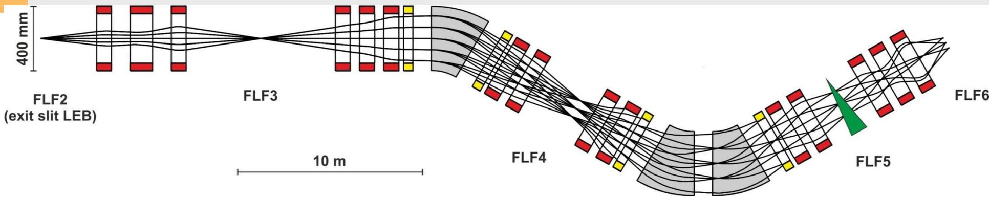
**The energy buncher at the low energy branch allows to fill the cryogenic stopping cell serving the low energy experiments MATS and LASPEC**
