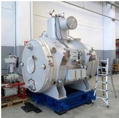
Copper plating and first tests of the RFQ accelerator cavity for the pLinac have been completed and match specifications
