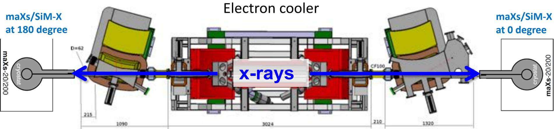
Two microcalorimeters, each at a distance of roughly 3 m from the electron cooler region.
